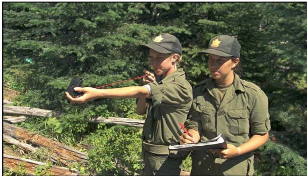
Figure 16-6-8 Taking a Magnetic Bearing
